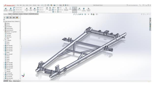
The above image shows one half of the chassis in standard form, and the other as a modified configuration to fit the bodywork.
